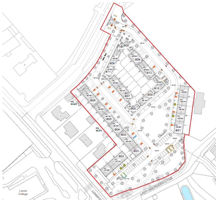
Fig 11: Waste management on site- orange rectangles indicate bin stores to front of dwellings
