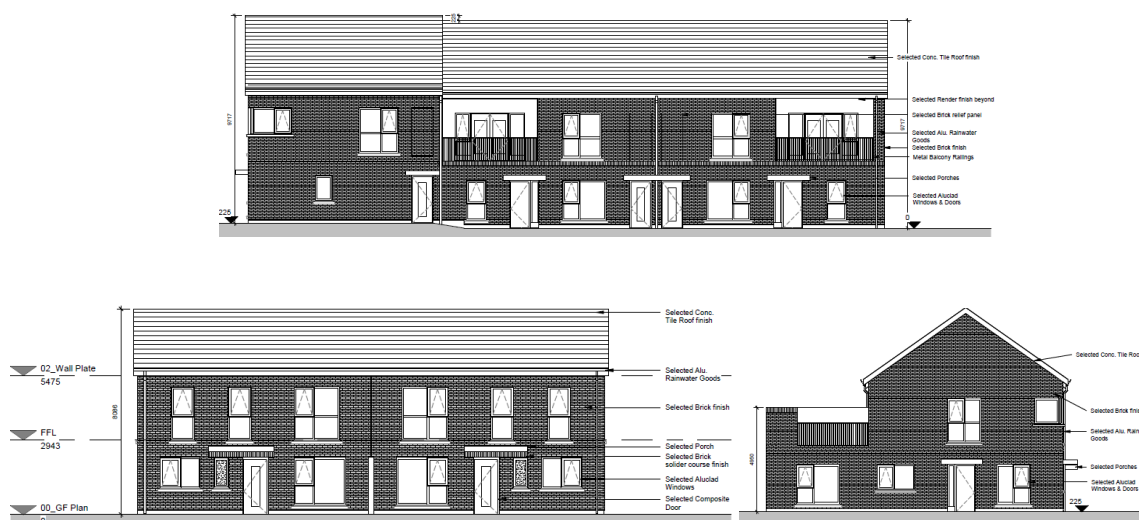
Fig 7: Typical Elevations of dwellings and duplex units
